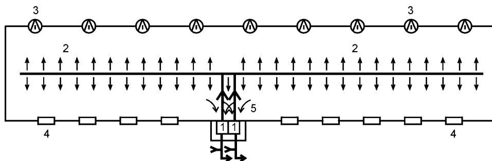
**Figure 1.** Animal house HVAC system flow chart: 1. Heat recovery exchanger of gravitation thermal pipes; 2. Foil sleeve for the distribution of heated outside air; 3. Axial fan; 4. Closable openings for the supply of atmospheric air; 5. Extraction of air from the animal house
