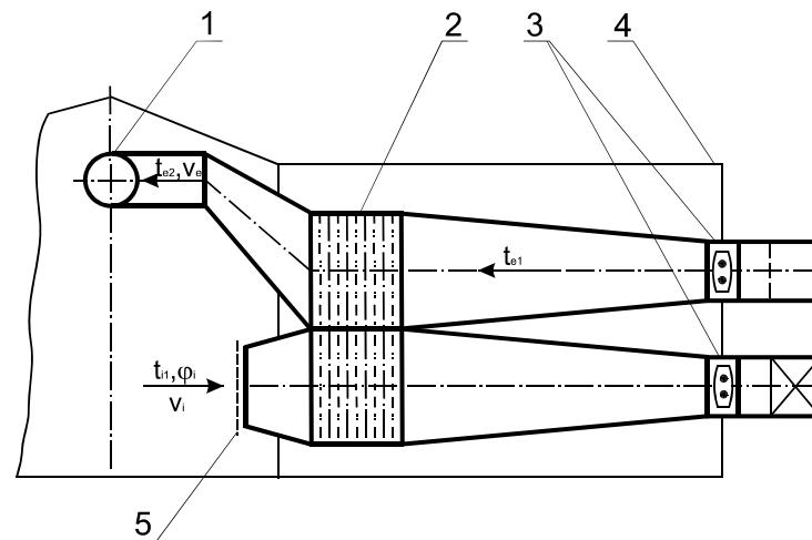
**Figure 2.** Drawing of the installation of the heat recovery exchanger and meters: 1. Foil sleeve for the distribution of heated atmospheric air; 2. Heat recovery exchanger consisting of thermal gravitation pipes; 3. Axial fan; 4. Annex for the heat recovery exchanger; 5. Filter
