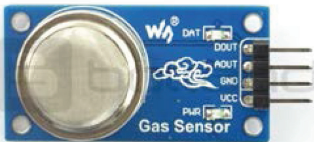
Figure 2. MQ-135 Carbon dioxide sensor (8)
