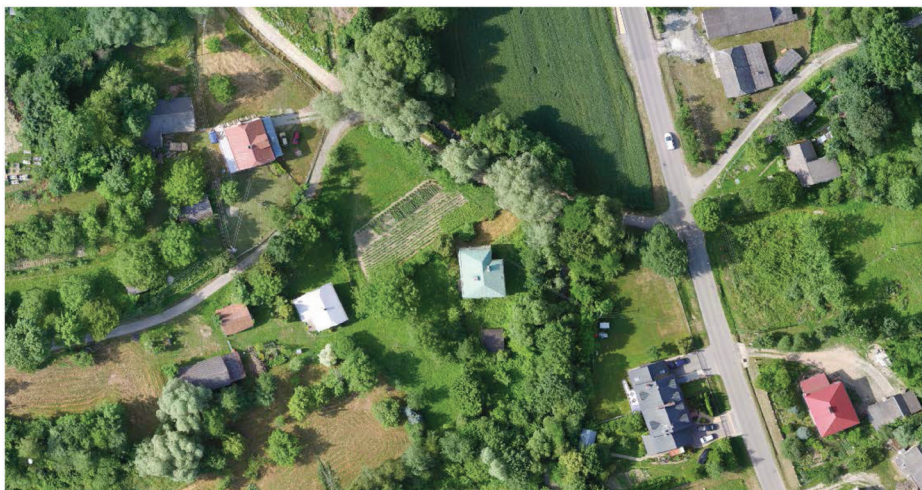
Figure 4. Digital orthophotomap of the landslide: pixel size (ground sampling distance) = 0.027 m
