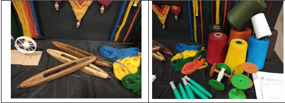
Figure 5. Tools and raw material (Fly shuttle, pirn, yarn etc)
